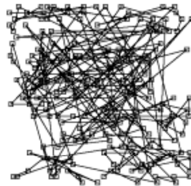
Figure 1: Power-driven scan chain routing on circuit s9234 without routing constraint
