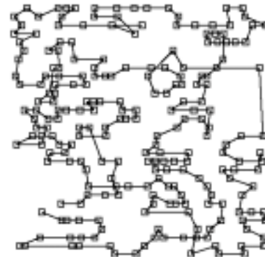
Figure 6: Scan chain routing on circuit s9234 obtained with “Silicon Ensemble”
