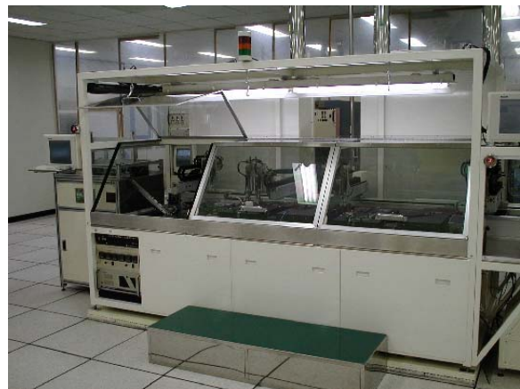
Figure 3. Baseline accelerometer test cell with linked tri-temperature test capability.
