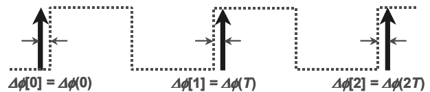
Figure 1. Illustration of timing jitter.
